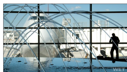
Fig. 2. Laminar jet fountain at the Detroit Metro airport (Courtesy of Wet Design).
