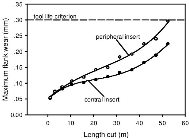
**Fig. 3** Typical progression of the maximum width of the flank wear land when using cermet central and peripheral inserts
