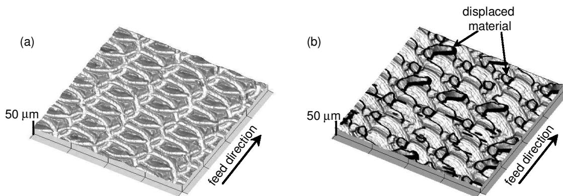
**Fig. 7** Three-dimensional topography of surfaces ( $2\text{ mm} \times 2\text{ mm}$ ) machined with (a) a new carbide tool and (b) a worn carbide tool ( $0.3\text{ mm}$  maximum flank wear)
