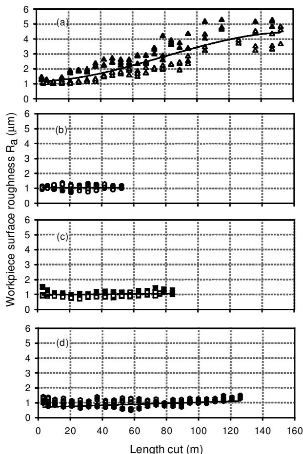
**Fig. 2** Transverse workpiece surface roughness versus length cut characteristics for the various insert combinations tested (the solid symbols refer to replicated experiments): (a) tungsten carbide central and peripheral inserts; (b) cermet central and peripheral inserts; (c) composite tool with cermet central and carbide peripheral inserts; (d) composite tool with relieved central insert and carbide peripheral insert
