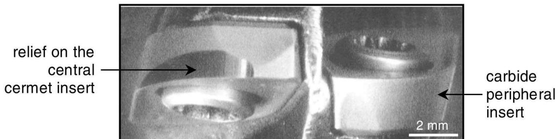
**Fig. 5** End view of the ball nose endmill, showing the relief provided on the central cermet insert to transfer
