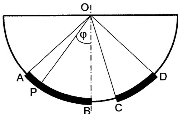
Fig. 6 Schematic of the indexable insert ball nose endmill, indicating the central (segment AB) and peripheral (segment CD) inserts
