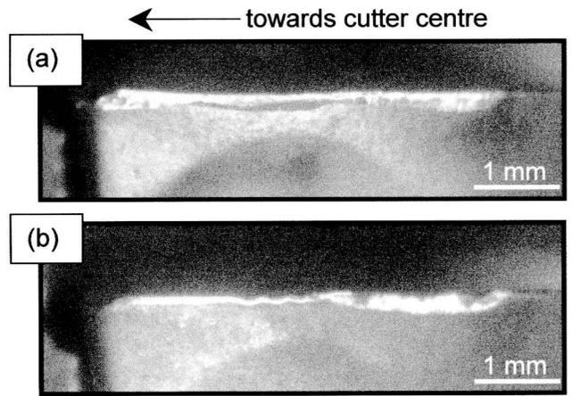
**Fig. 4** Representative flank wear patterns on the central insert: (a) tungsten carbide; (b) cermet
