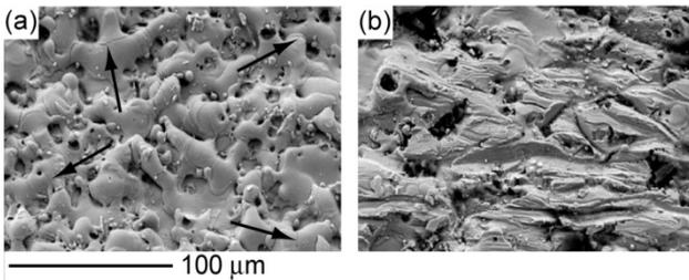
Figure 7: Machined surfaces from: (a) WEDM, (b) AWEDM.
