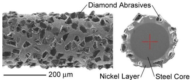
Figure 3: Surface and section of diamond wire.
