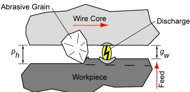
Figure 2: The interelectrode gap in AWEDM.
