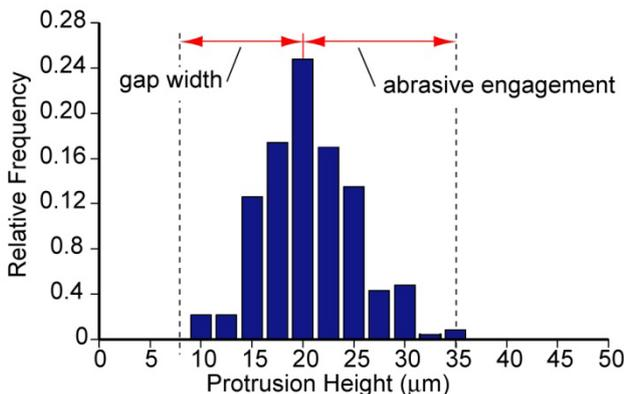
Figure 4: Protrusion height distribution of abrasive wire.
