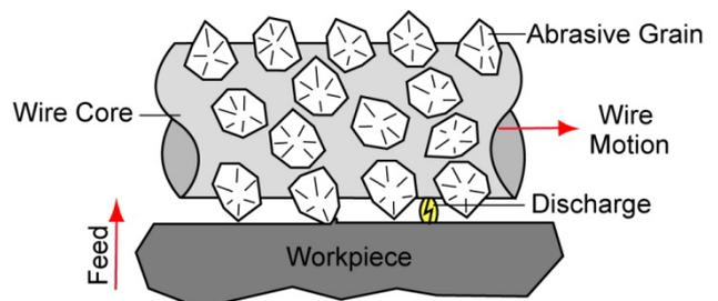
Figure 1: Schematic of AWEDM.
