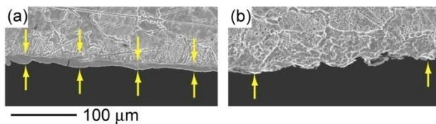
Figure 8: Sectional view of surfaces machined using: (a) WEDM, (b) AWEDM.
