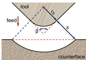
Fig. 1. Schematic representation of electro erosion edge honing.
