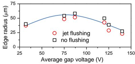
Fig. 6. Effect of gap voltage and flushing on edge radius.
