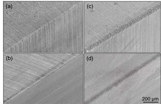
**Fig. 4.** Micrographs of: (a) HSS and (b) cemented carbide ground (sharp) edges; (c) and (d) are the corresponding electro-erosion honed edges.
