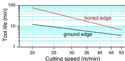
Fig. 7. Effect of edge preparation on tool life.
