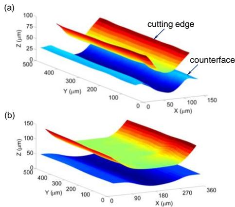
**Fig. 2.** Effect of counterface material on edge geometry: (a) aluminum, (b) copper.
