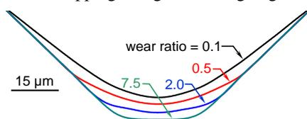
**Fig. 3.** Simulated effect of wear ratio on edge geometry.
